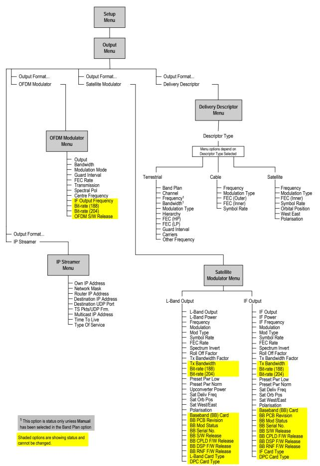
Figure 4.17: Menu Hierarchy – Setup/Output Menu
